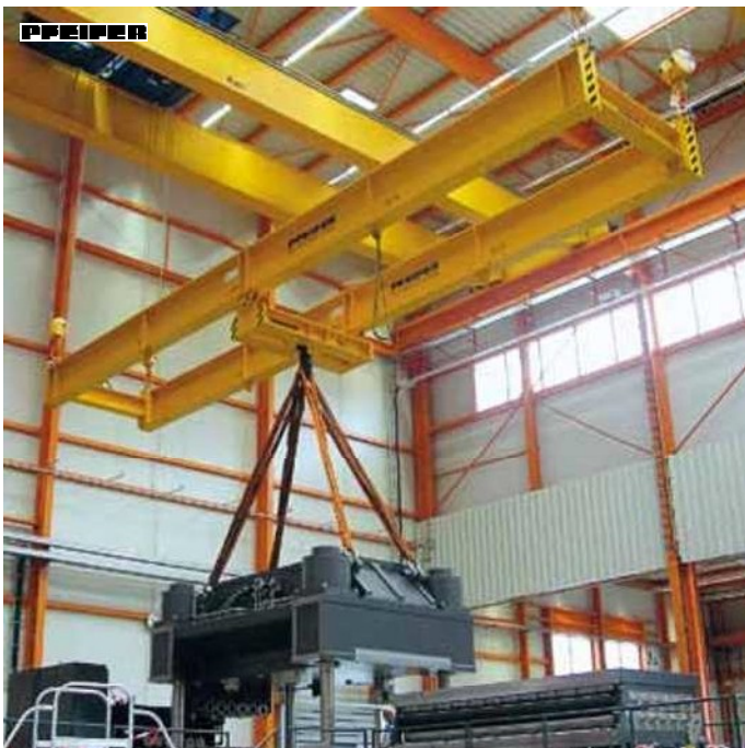
Crane lower blocks 75 t 4 pulleys with electrically revolving hooks
