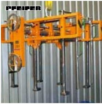
Grab for Sheet-Blanks 3.8 t for transporting stacked metal-sheet blanks
