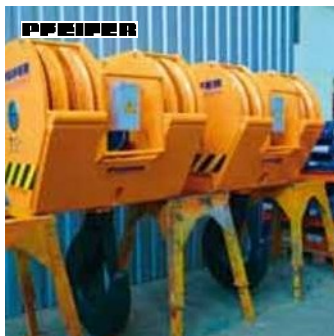
Crane lower blocks 75 t 4 pulleys with electrically revolving hooks
