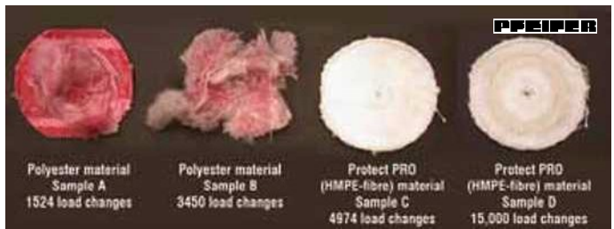
The abrasion of Protect PRO (HMPE-fibre) compared to polyester
