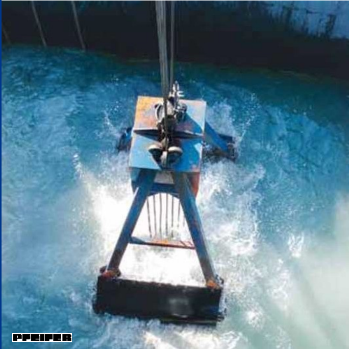
Grab dredgers: Ropes raise, lower and close the grabs
