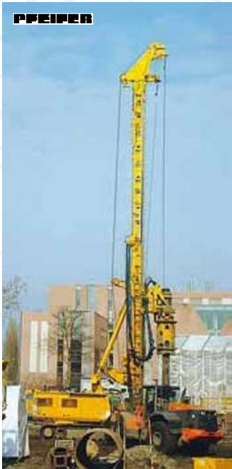
Rotary drilling rigs: Ropes raise and lower the drill rods
