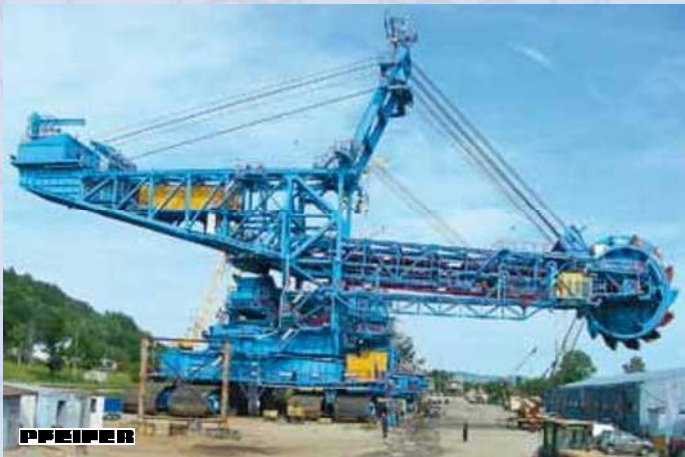
Open-cast mining excavator: Ropes hold and move the booms
