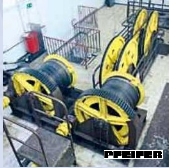
Container gantry cranes: Ropes raise and lower the spreader for transporting the containers
