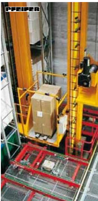
Shelf-operating devices: Ropes raise and lower the lifting platform and the transfer unit
