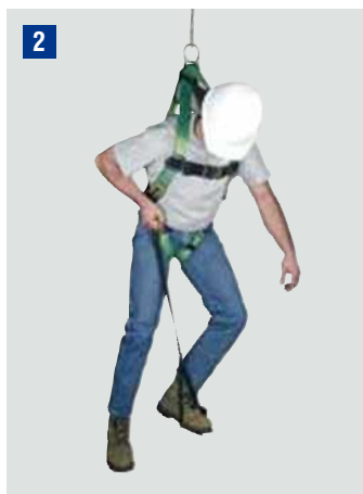
2 Step into the step sling and adjust the length.
